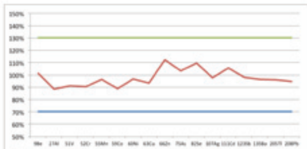
Figure 6. Laboratory fortified matrix minor & trace element recoveries (Method specified 70 – 130% limits shown)
