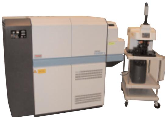
Figure 3: Finnigan ELEMENT 2 with New Wave UP213 laser system.
