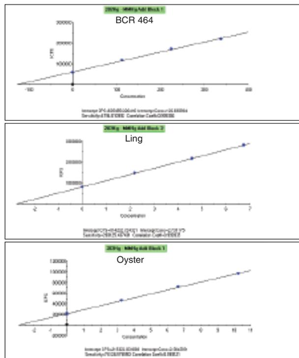
Figure 4: PlasmaLab Standard Addition curve for BCR 464, Ling and Oyster samples
