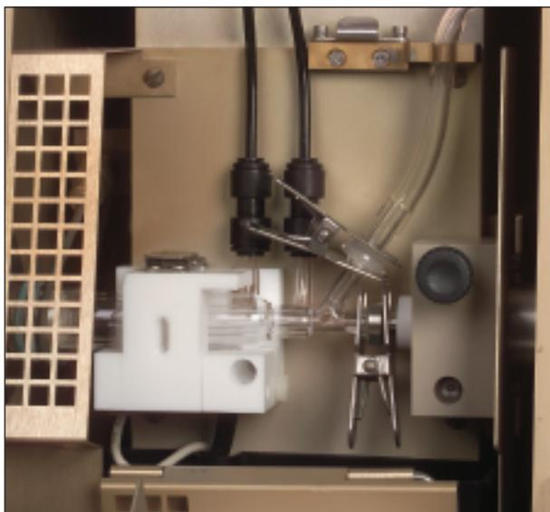
Figure 2: X Series dual mode sample introduction for GC-ICP-MS
