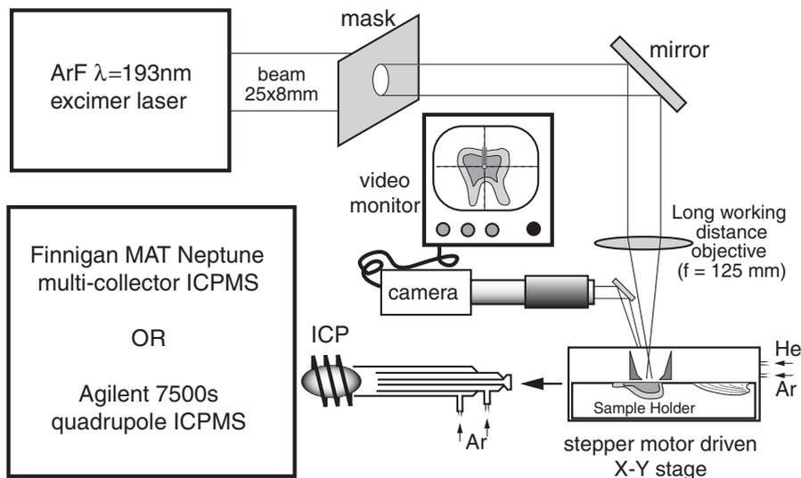
Fig. 1. Schematic diagram of the ArF ( $\lambda = 193$  nm) excimer, laser ablation multi-collector ICPMS system used at the Australian National University.
