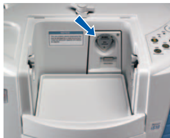
The Nicolet iS10 source is mounted in the sample compartment allowing quick and easy optimization of data collection in the mid-near or infrared region.
