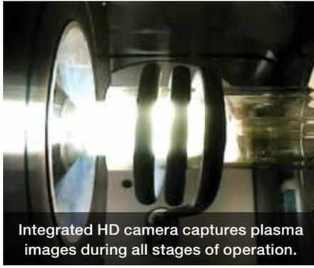
Integrated HD camera captures plasma images during all stages of operation.
