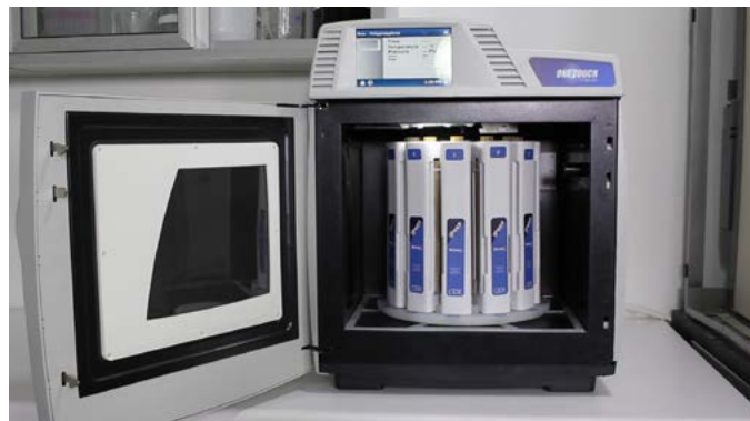
MARS 6 Microwave Digestion System, with iWave Light Emitting Technology and iPrep vessel turntable
