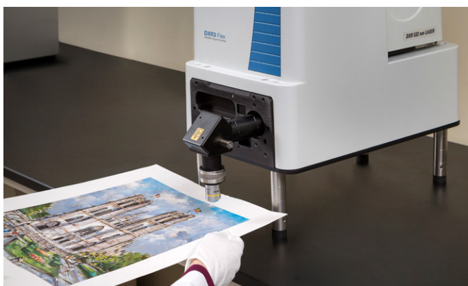
DXR3 Flex Raman spectrometer equipped with a microscope accessory for art authentication analysis.
