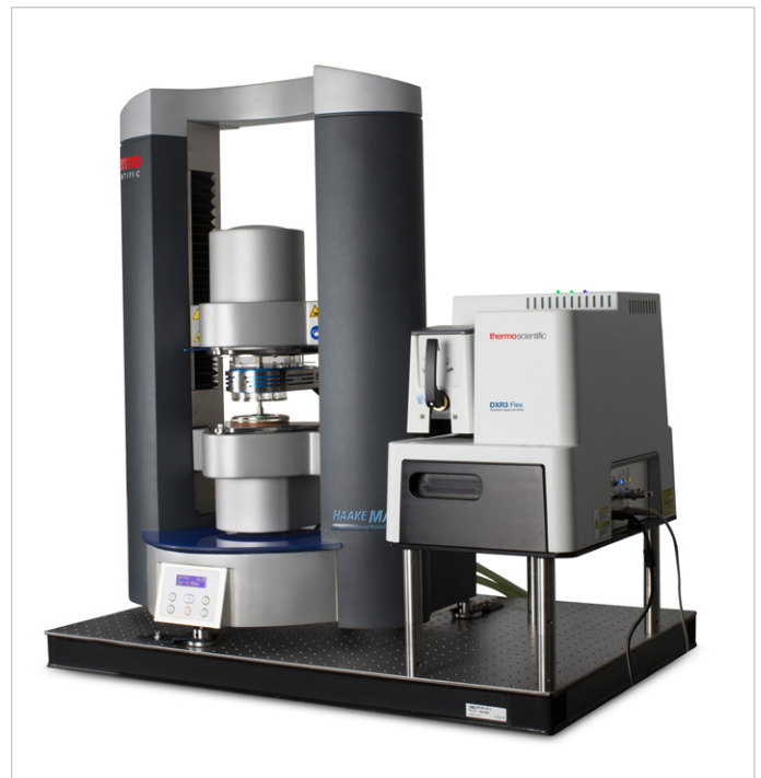
DXR3 Flex Raman Spectrometer integrated with a Thermo Scientific HAAKE™ MARS™ Rheometer.
