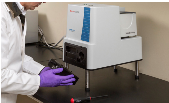
DXR3 Flex Raman spectrometer being outfitted with a user-replaceable macro sample measurement accessory.
