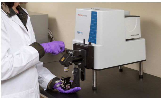
DXR3 Flex Raman spectrometer equipped with micro-stage sampling accessory for point-and-shoot measurement.
