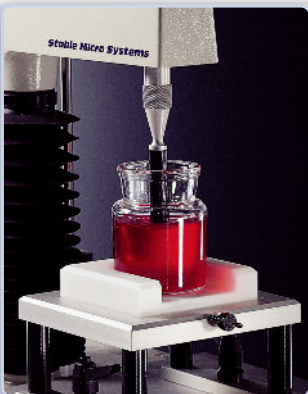
0.5" Diameter Cylinder Probe With the use of a Bloom Jar and Centralising Base. For GMIA or ISO Standard Bloom Strength (Gelatine) or Gel Strength measurement.
