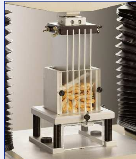
Figure 5: A Kramer shear cell is typically suited to meat pieces or coated meat products
