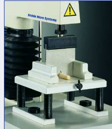
Figure 3: “Standard” Warner Bratzler shear force test
