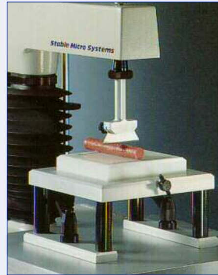
Figure 8: Razor blade shear force can be assessed using a readily available craft knife attached to a TA.XTplus Texture Analyser
