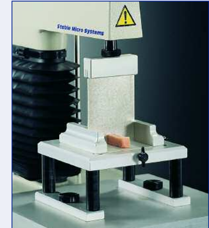
Figure 4: “European” Warner-Bratzler “Standard” blade for Meat testing
