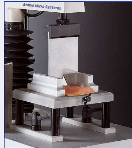
Figure 1: A Stable Micro Systems Warner-Bratzler blade (stainless steel, 70mm wide, 90mm high, 3.2mm thick)
