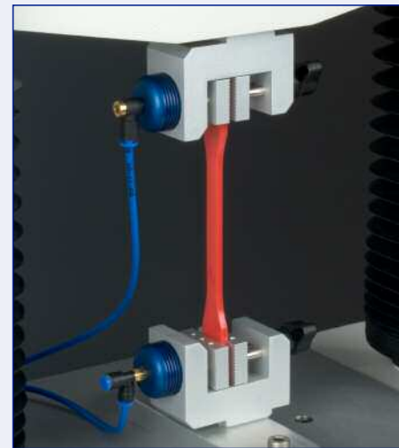
Figure 16: Measurement of tensile properties of meat – samples clamped via Pneumatic Grips
