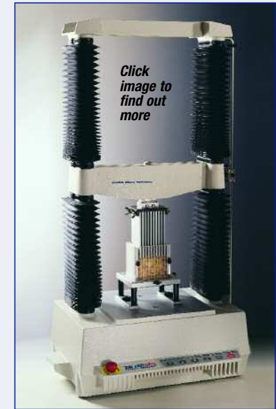
The TA.HDplus Texture Analyser – required for high force texture analysis
