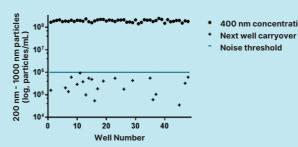
Particles >200 nm measured using a NanoSight NS300 with Sample Assistant, detected in particle-free water wells positioned subsequently to wells containing 400 nm polystyrene standards. There was an average carryover of 2 particles per 10 frames of video captured by NTA software – well below the standard noise threshold.
