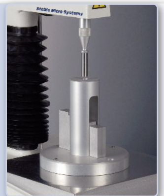
Low Tolerance Powder Compaction Rig* Suited to powder compaction applications where the punch/die clearance is less critical.
