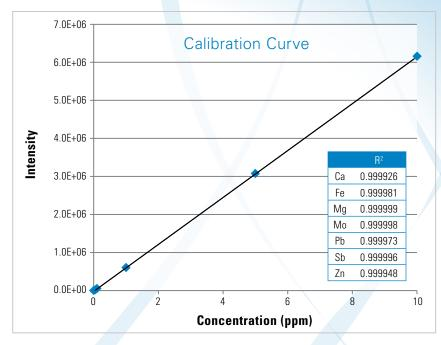
**Standard Preparations** – The SimPrep can prepare the entire curve from a single stock solution. This brings a high level of precision and accuracy to the most important prep of the day. Don't worry about the analyst on duty or the day of the week, get the same prep every time. Autocalibration data from a 6 point curve. Standards prepared from a 100 ppm stock at 10× to 2000× dilution.
